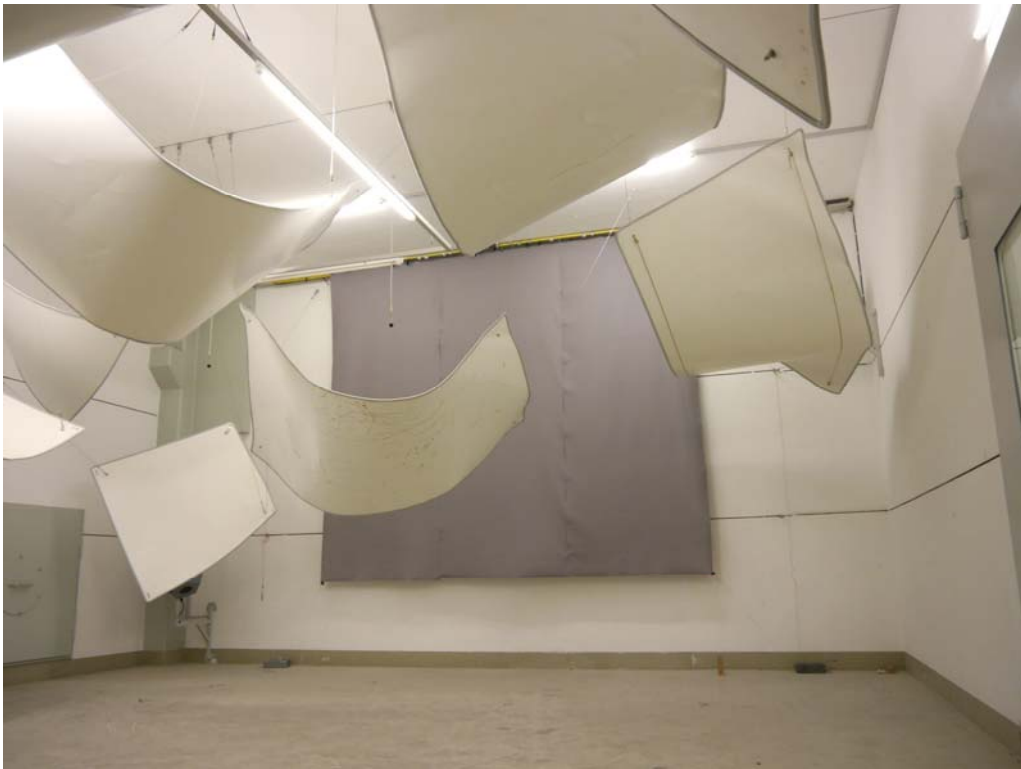
Figure B1. Flat arrangement, test object mounted in the reverberation room.
